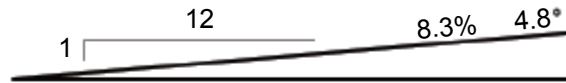
Standard Ramp - 1 in 12 "A foot of ramp for each inch of rise"
